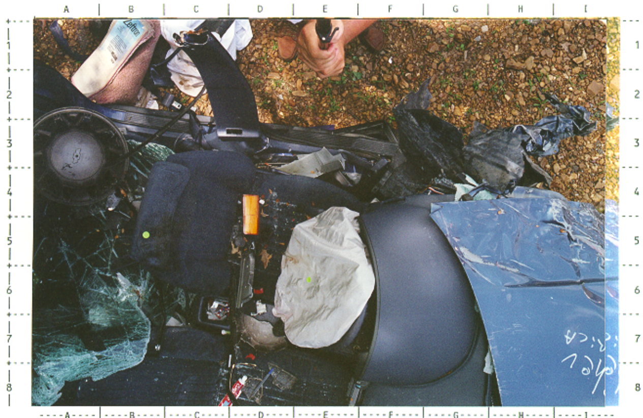
# 40 -- Overhead left center view of 1991 Chevrolet Corsica's driver area; NOTE: deployed air bag & roof peeled-back for extraction
